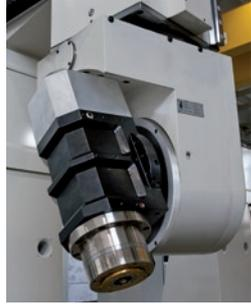
T2D-04 head with HSK-A-63 spindle
