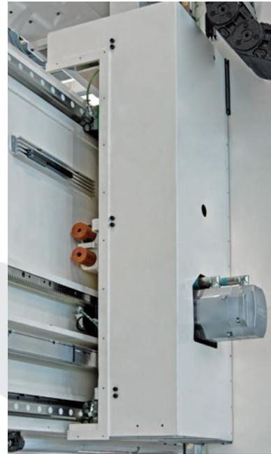
Cross axis frame (Y axis) composed of an electrowelded steel crossbeam with two preloaded roller guide-ways for Y-axis saddle movement
