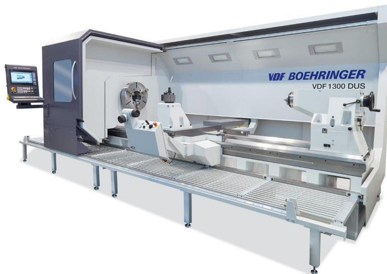
The new model size VDF 1300 DUS is designed for reliable large part machining with high rigidity and long term precision.
