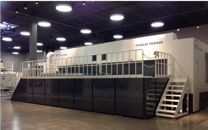
The SNK 5-axis profiler HPS-120A is a rigid and powerful machining center for tough metal cutting jobs, including titanium milling.
