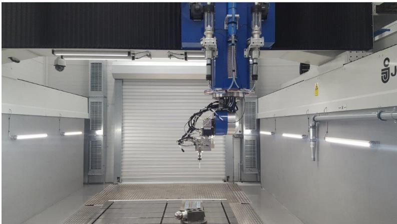
Jobs Laser Speeder: an additive manufacturing machine equipped with laser head. The system is conceived to perform cladding, hardening and measuring operations on very large dies for the automotive field.
