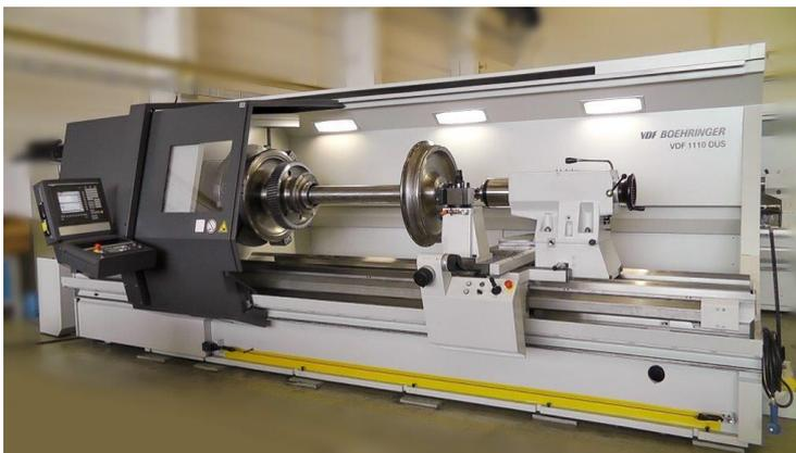
VDF Boehringer lathes and turning centers cover a full range of railway applications, from wheelset or wheel repair to production of new axles.
