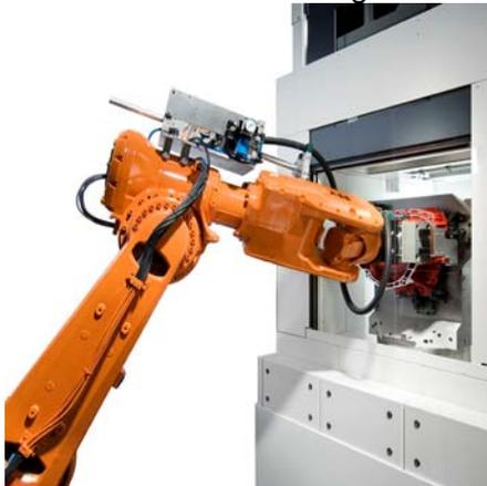
core of the setup. A gantry-mounted robot is used for loading parts and tools into the machine or pallet changer. These are supplied by an automated guided vehicle (AGV), which can generally be equipped with any kind of workpiece carrier and robot coupling. The part
