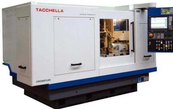
Tacchella Crossflex – the grinding experts from Cassine/Italy will present an external cylindrical grinding machine with in process gauge and flexible automation possibilities
